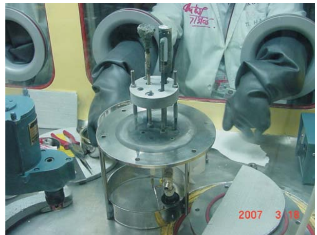
Fig. 1 : Electro-refining cell inside glove box
