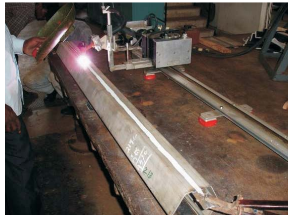
Fig. 1 : Photograph of A-TIG welding under progress in hexagonal sheath
