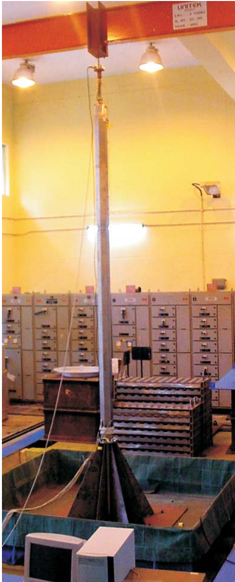
Fig. 3 : Test setup mounted on the shake table
